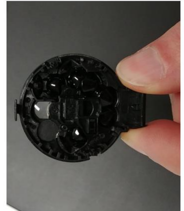
Figure 2. Left: Rain measurement principle. Right: Rain channel NIR light-guide optics and transparent global sun optics
